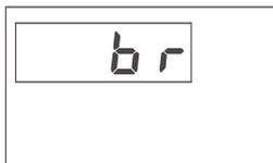
**br** broken probe or input values higher than maximum limits
