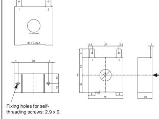
These transformers are used to measure current at 50 ÷ 60Hz from 25A at 600A (rated primary current lp). The special characteristic of these transformers is the high number of turns of the secondary (Is). This produces a very low secondary current, appropriate for an electronic measurement circuit. The secondary current can be read as voltage on a resistor.
