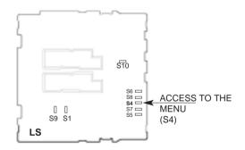
Jumper S4 is normally closed. To change its state, the connection has to be removed. This operation must be done by trained technical personnel.
