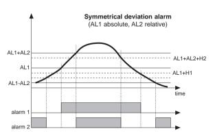
For AL1 direct absolute alarm (max) with negative H1, 1 t = 0 For AL2 symmetrical deviation alarm H2, 2 t = 6
