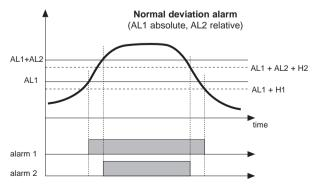
For AL1 direct absolute alarm (max) with negative H 1, 1 t = 0 For AL2 direct relative alarm (max) with negative H2, 2 t = 2
