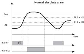
For AL1 inverse absolute alarm (min.) with positive H1, 1 t = 1 (\*) = OFF if disabling on power-on exists
