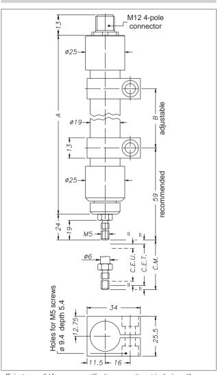
Important: all the data reported in the catalogue linearity, lifetime, temperature coefficient are valid for a sensor utilization as a ratiometric device with a max current across the cursor Ic  $\leq$  0.1  $\mu$ A
