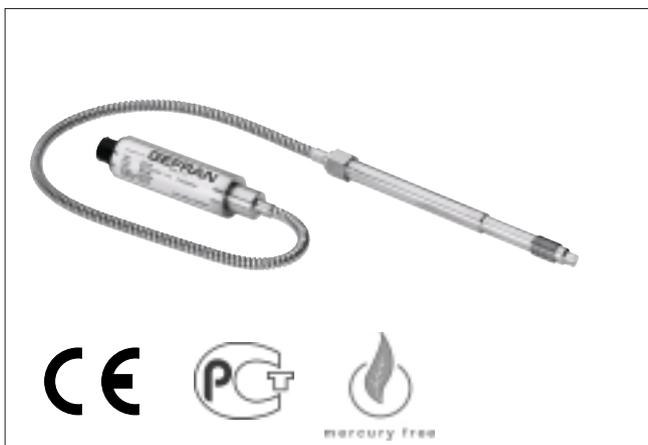
The K3 Series are for use in high temperature applications where the process temperatures may reach 538°C (1000°F) such as high temperature engineered polymers. The K Series utilizes standard melt pressure principles and construction, but uses a near incompressible NaK (Sodium Potassium) for pressure transmission. The K Series strain sensing technology is bonded foil strain gage.
