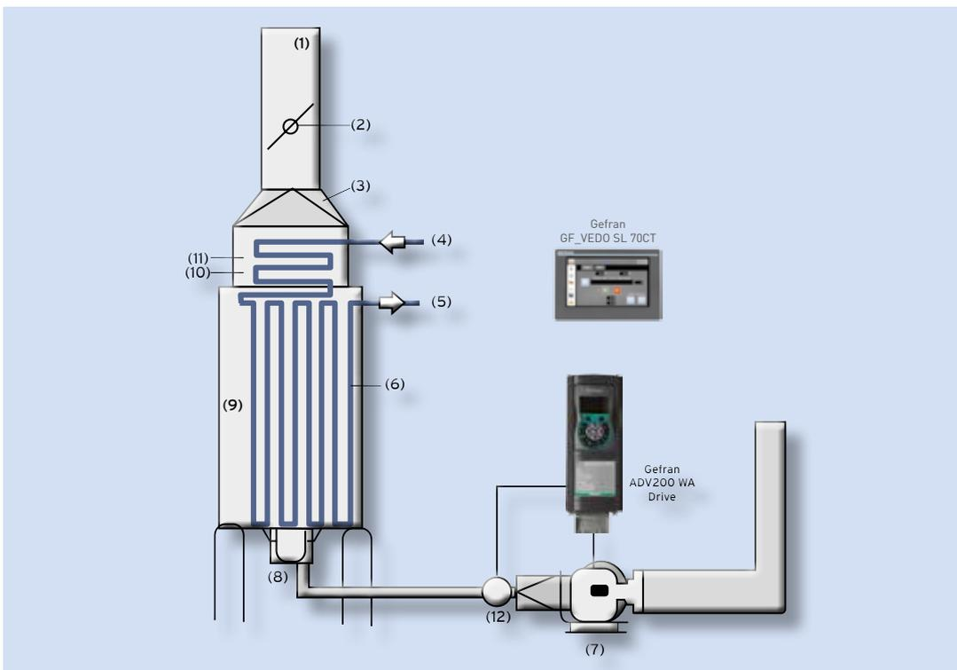
*By means of the PID controller, the ADV200WA manages the air flow required by the process.*
