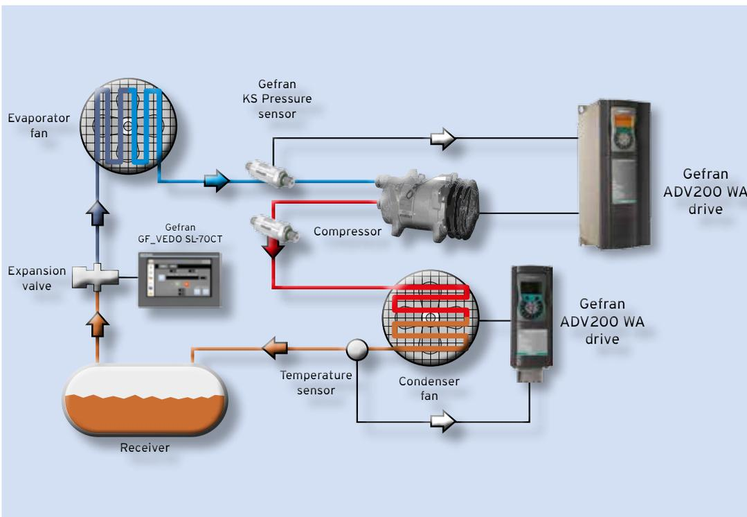
*The drive controls compressor speed in accordance with a pressure setpoint.*
