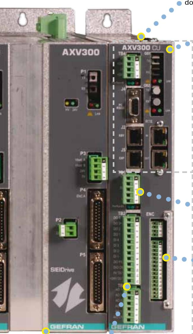
**SD-card** for storing configurations and downloading system data
