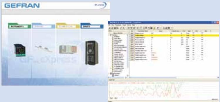
All drives in the SIEIDrive range and automation devices manufactured by the GEFRAN group (PLC, HMI, instrumentation, etc.) can be programmed via PC using the **GF\_eXpress** configurator, a programming environment that enables complete setup and control of the product, based on a powerful, user-friendly and intuitive software platform:
